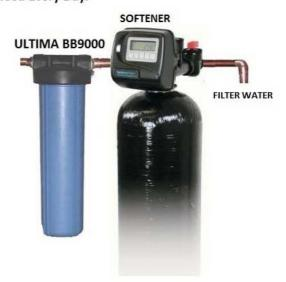
The Ultima BB9000 sediment pre-filter system reduces particulates in the supplied water down to 5 micron (20 times smaller than a human hair) in size. Routine replacement of this 5-micron sediment filter will increase the effectiveness and protect plumbing and appliances from excess sediment. With average use, each filter is effective for approximately 6-12 months. The unit comes in 3 colors, solid white, blue and black.
